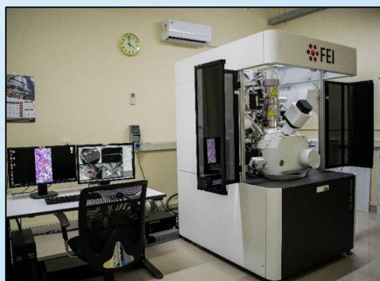
Dual Beam System (Helios G4 UX) at NFAPT, IIT Madras
